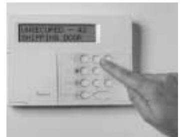
The KP103 Keypad's backlit readout displays system status.
